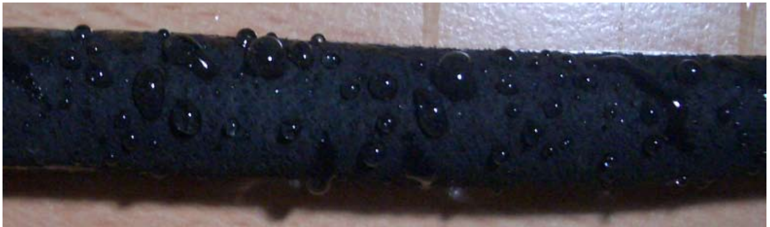
One part of hose when water is injected (With mini Water Pressure)
